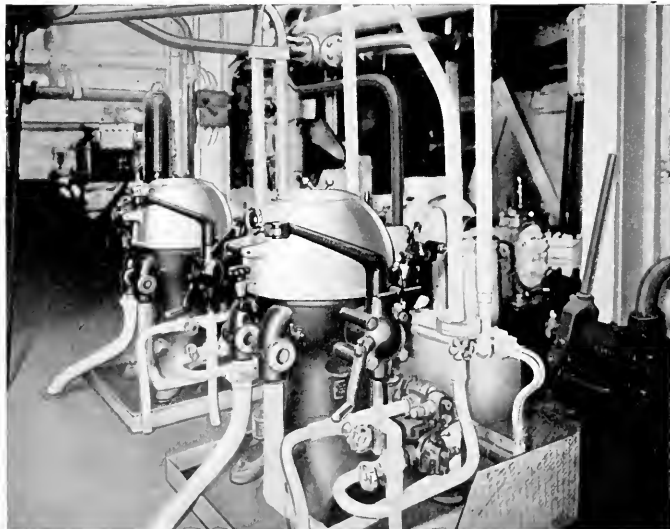
Above, motorship and whale oil factory Sir James Clark Ross. At left, the two totally enclosed vapor-proof De Laval fuel oil purifiers serving the main engines of the Sir James Clark Ross.
